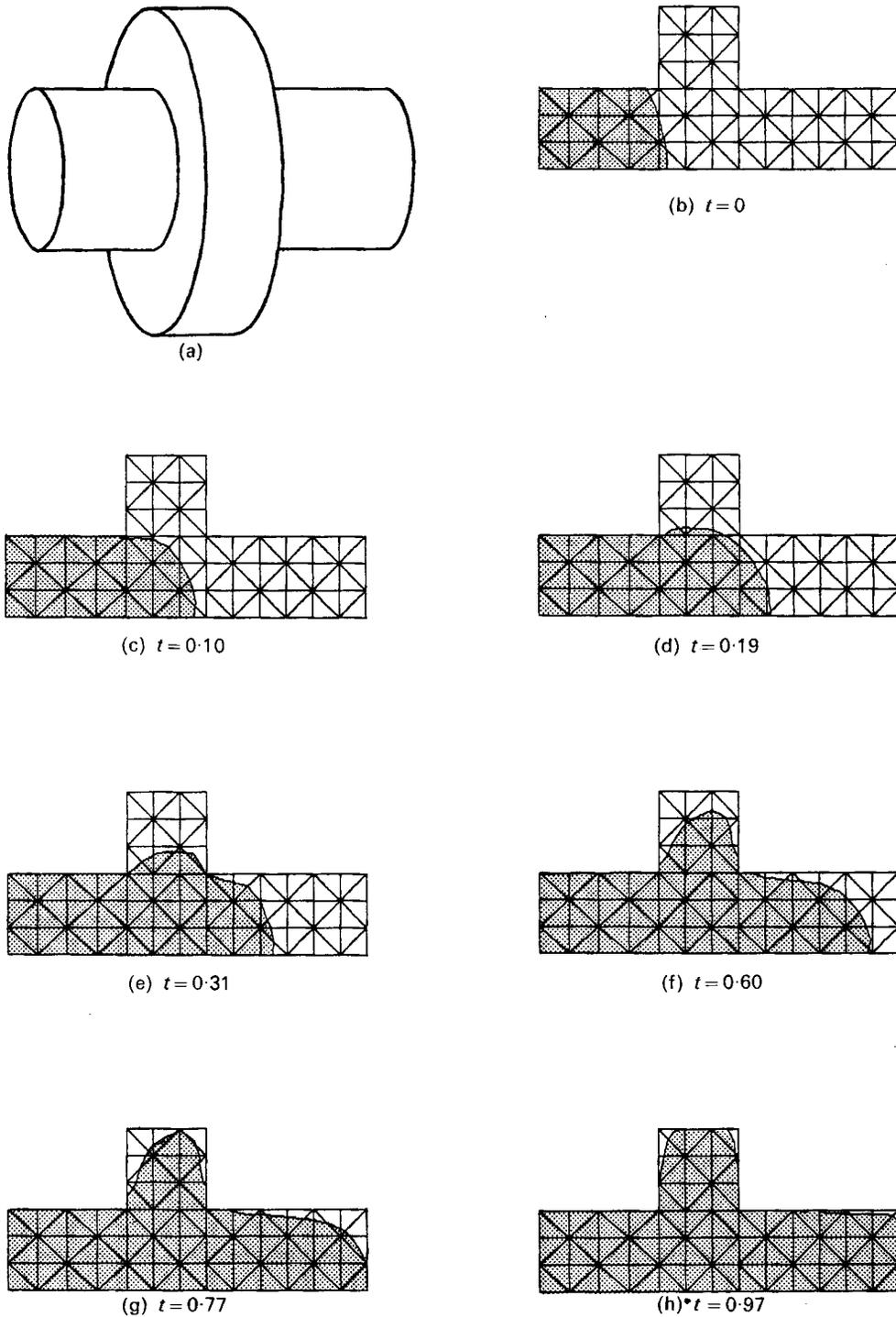
Figure 1. Axisymmetric analysis of the flow of fluid during injection moulding: (a) shape of mould; (b)–(h) profiles of the fluid as the mould is filled
