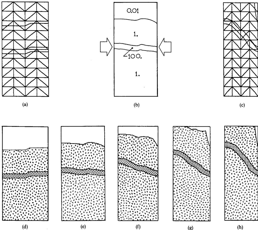
Figure 8. Deformation of rock strata during compression: (a) initial mesh with critical contours; (b) relative viscosities of the rock; (c) final mesh with critical contours; (d)–(h) deformation of the strata during compression
