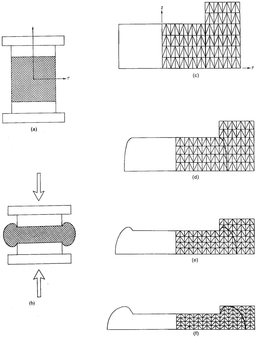
Figure 2. Compression of a cylindrical specimen: (a) geometry of the problem at the start of analysis; (b) final shape of the specimen; (c)–(f) deformation of the specimen during forging
