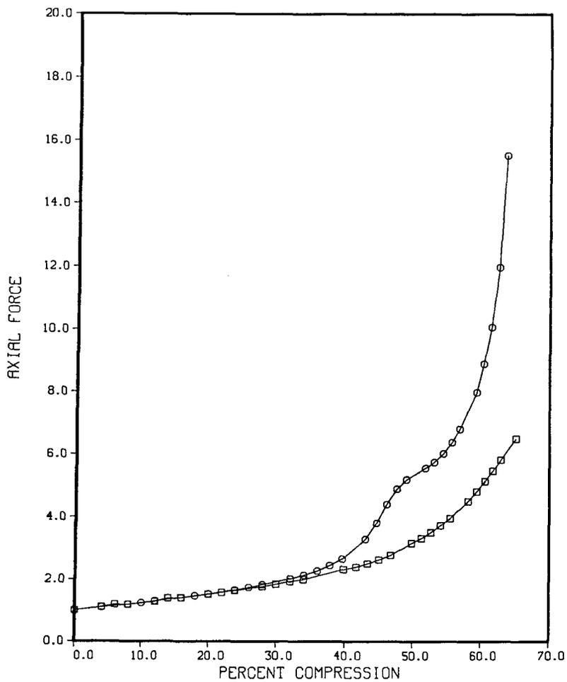
Figure 4. Axial force during compression. Quasi-Lagrangian analysis represented by circles, pseudo-concentration analysis represented by squares
