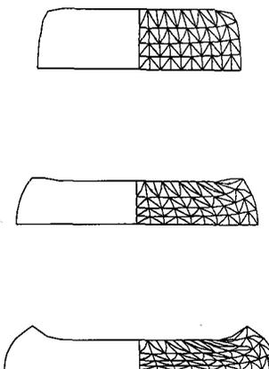
Figure 3. Deformation of specimen and mesh during a quasi-Lagrangian analysis
