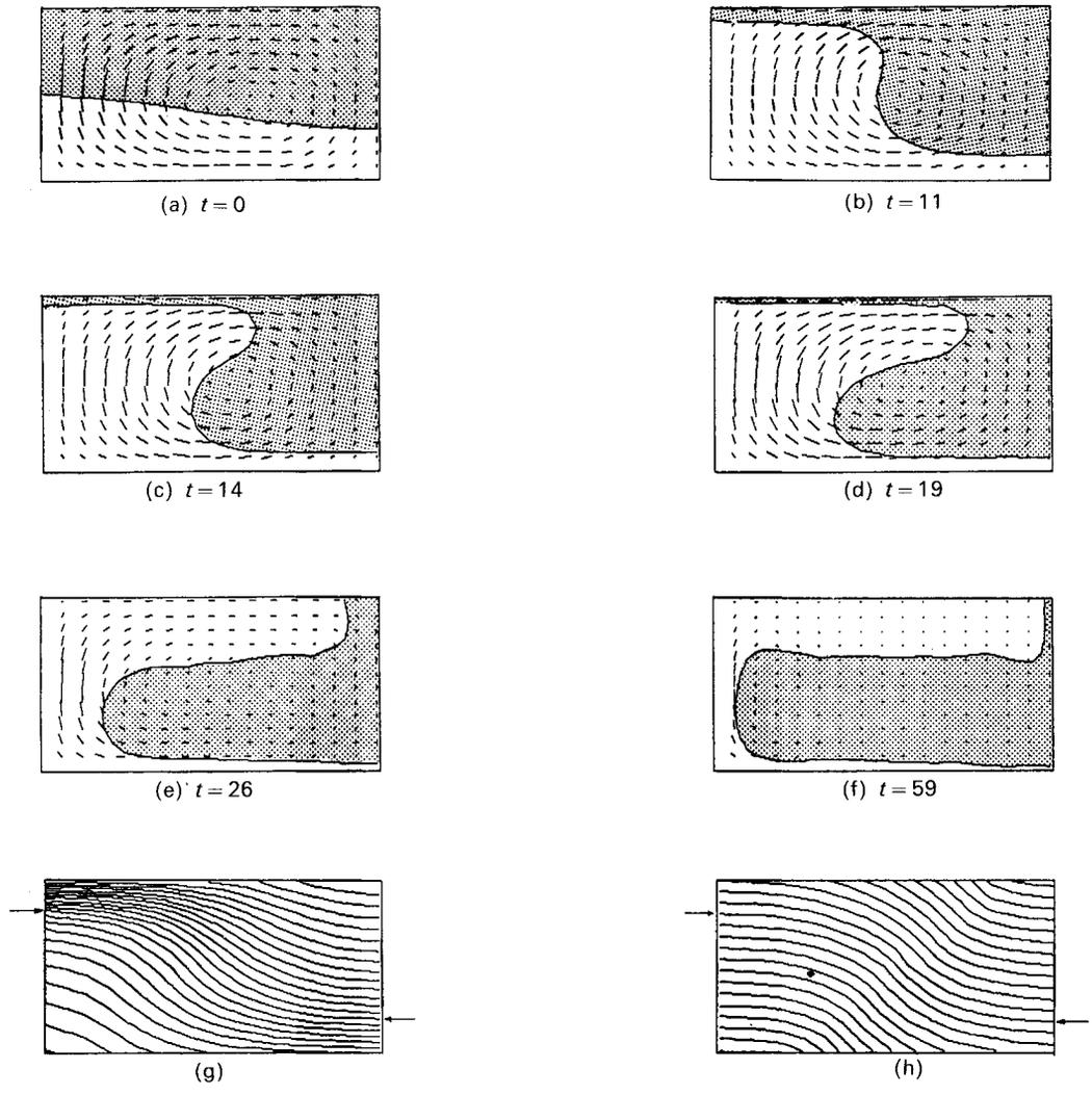
Figure 7. Solution to the convective flow problem: (a)–(f) convective flow patterns showing velocity vectors and the interface contour; (g) *M*-surface contours before smoothing; (h) *M*-surface contours after smoothing
