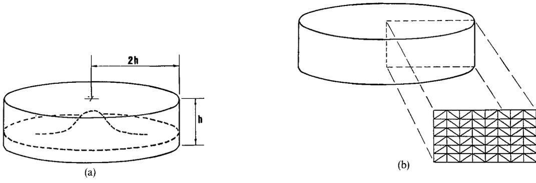
Figure 6. Convective flow of two fluids in a closed container: (a) physical layout showing lighter fluid rising at the centre of the container; (b) finite element mesh used for analysis
